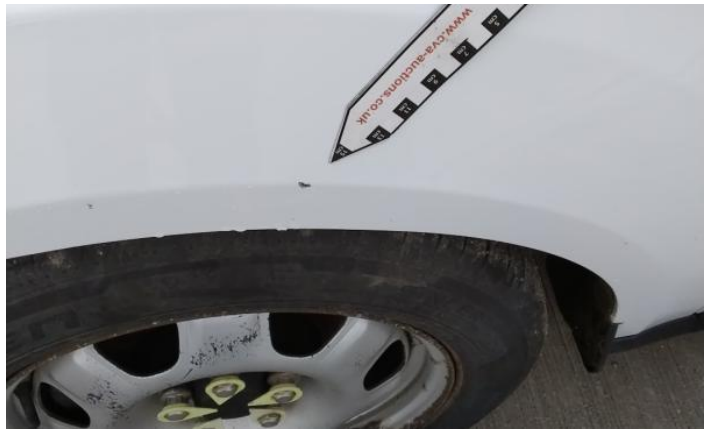
4: Wing nsf Chipped Multiple Chips
