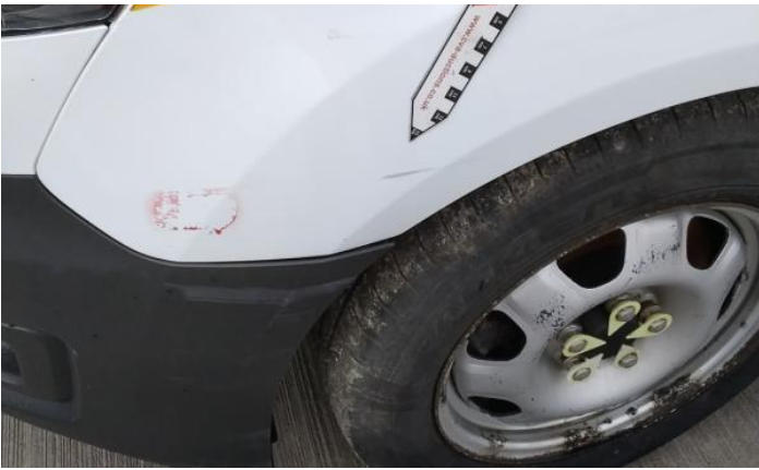
3: Bumper Front Scratched Over 100mm Thru Paint
