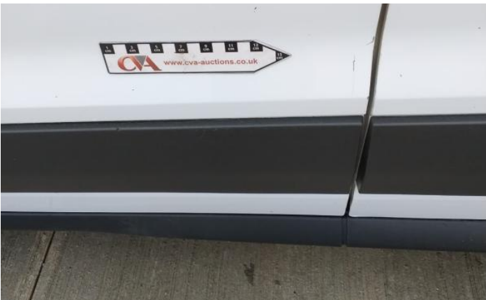
5: Wing nsf Scratched Over 25mm Thru Paint
