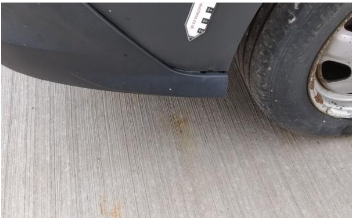
11: Bumper Rear Scratched Over 100mm Thru Paint
